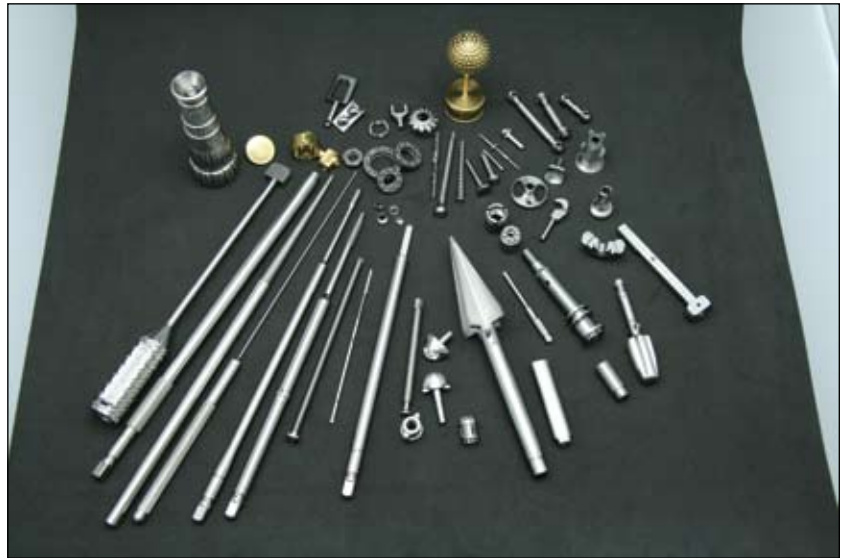
◀ Some of the parts C&A produces on Swiss machines using PartMaker programming.
